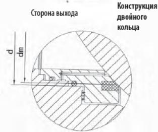
3) FIRST AID OF SEAL The valve is designed with an auxiliary seating emergency seal system, as shown in the figure. In case of soft seal damaged, or failure of seal in an emergency circumstances, emergency seal may be effected by injecting in sealant through auxiliary sealing system. If needed, emergency seal assembly can be used to rinse and lubricate the seating area. Plus, valve stem can also be designed with an auxiliary emergency sealing system.
