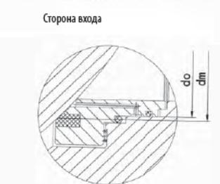
4) FIRE PROTECTION STRUCTURE If requested by working conditions and users, ball valve may be designed to fireproof. The fireproofing design of ball valve is to the standards of API 607 and JB/T6899. In case of soft seal ring burnt in fire, the fire protection structure of ball valve functions to prevent mediums from mass leakage, thus to avoid fire spreading.
