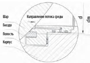
2) SELF-RELIEVING STRUCTURE In case of abnormal rise of pressure at middle cavity, ball valve of single seal structure is provided with self-relieving function, while ball valve of dual seal structure uses the auxiliary pressure relief device on valve body to carry out pressure relief.
